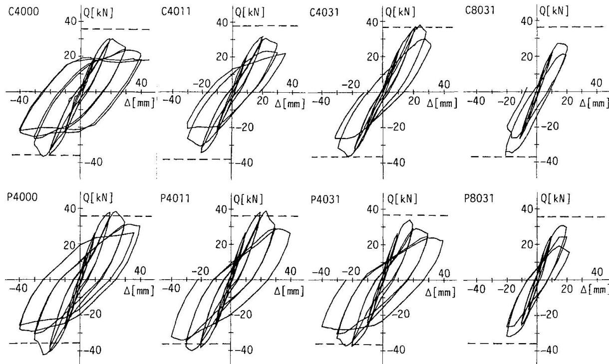
Fig. 3 Relations between Load  $Q$  and Displacement  $\Delta$
