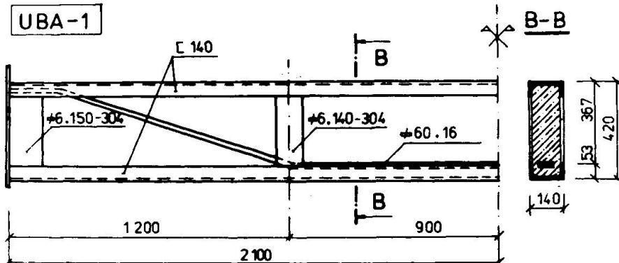
Fig. 2 Details of the beam UBA1
