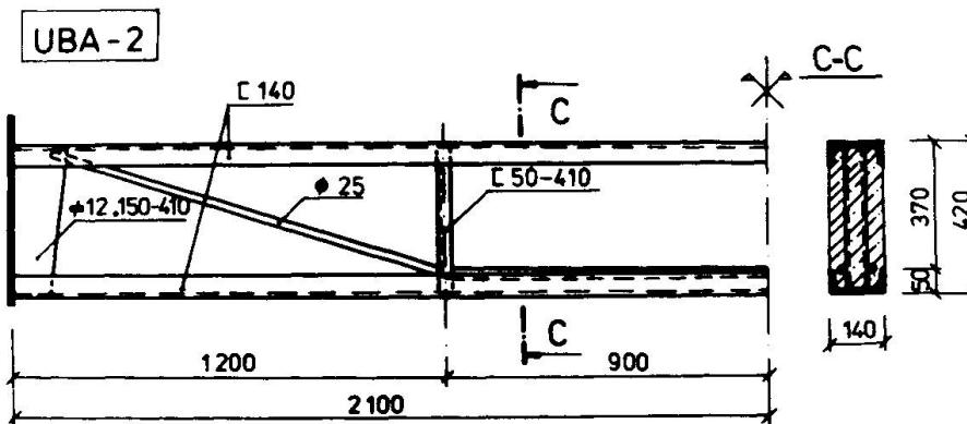
Fig. 3 Details of the beam UBA2
