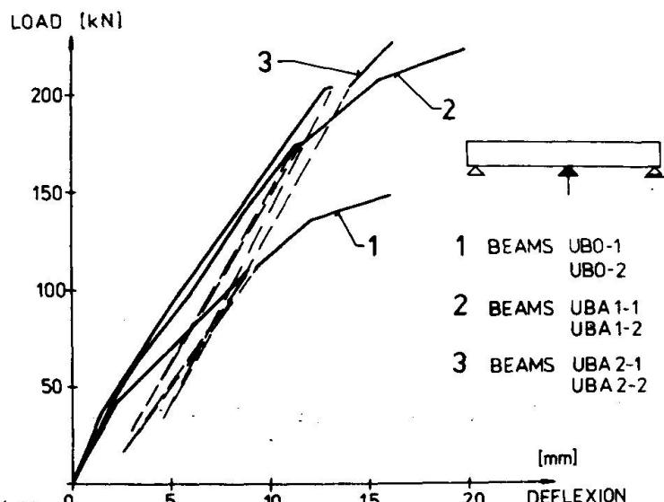
Fig. 4 Load-deflection curves for centre spans
