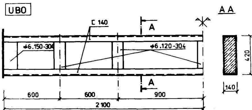
Fig. 1 Details of the beam UBO
