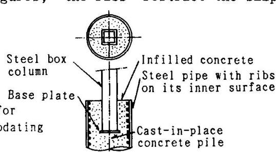
Fig. 2 Column-pile connection
