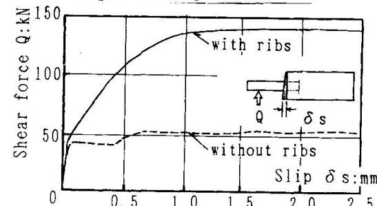
Fig. 5 Envelopes of load to slip-out of concrete curves (specimens with pipe 318.5φ)
