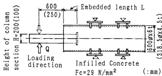
Fig. 4 Test specimen
