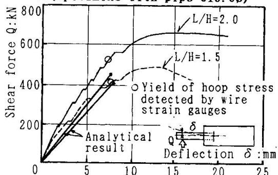
Fig. 7 Envelopes of load to deflection curve (specimens with pipe 600φ)
