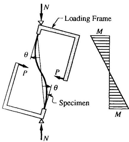
Fig.3 Loading setup and moment distribution of specimen
