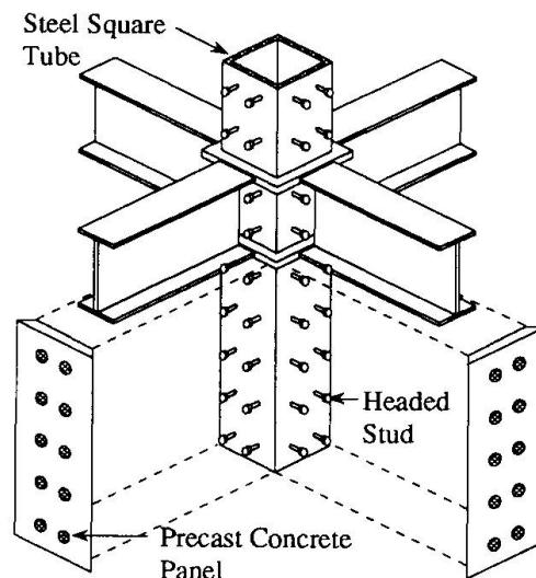
Fig. 1 The Concept of the Composite Column Structural System
