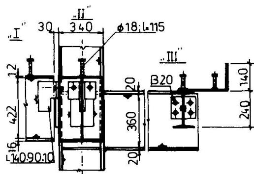
Fig. 2. Connection girders to column
