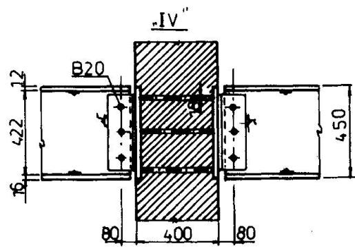
Fig. 3. Connection girders to concrete
