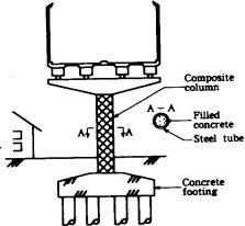
Fig.1 Bridge with composite column
