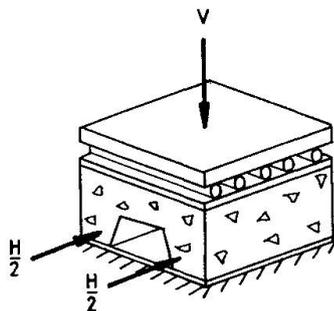
Fig. 1 Schematic Representation of Slip Block Test Set-up
