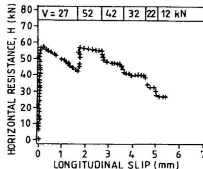
Fig. 3 Trial Slip Block Test Performed on Profile A Showing H-Slip Curve
