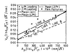
Fig. 1 Shear-Bond Plot of Test Results
