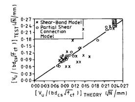
Fig. 5 Comparison of Test Results with Theoretical Predictions
