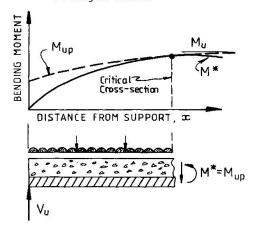
(a) Free-Body Diagram of Slab End Segment Bounded by Critical Cross-section
