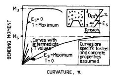
Fig. 3 Derivation of Composite Slab Moment-Curvature Relationships
