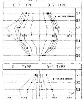
Fig.9 Distribution of shearing strain of steel member
