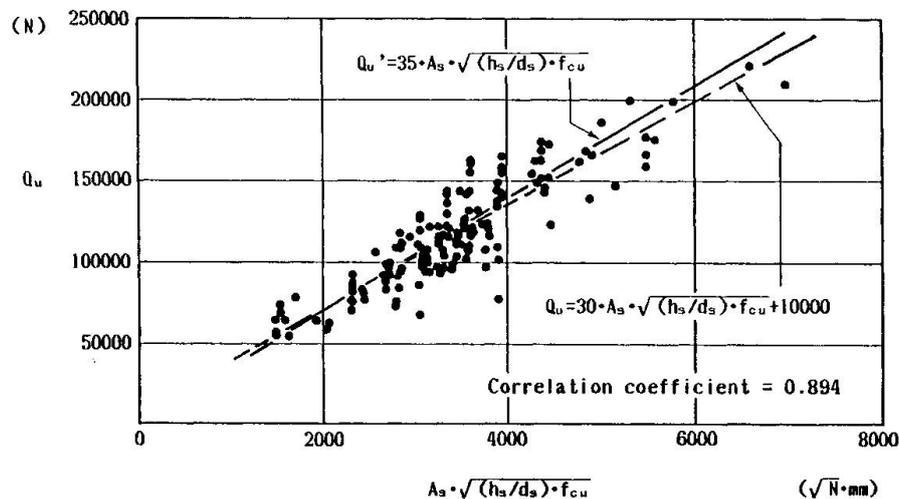
Fig. 3  $Q_u - A_s \cdot \sqrt{(h_s/d_s)} \cdot f_{cu}$  relation
