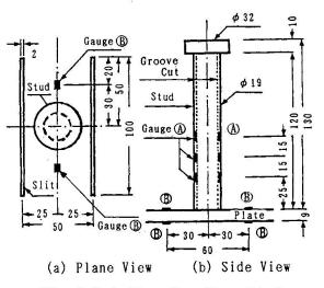
Fig.3 Details of a View Stud
