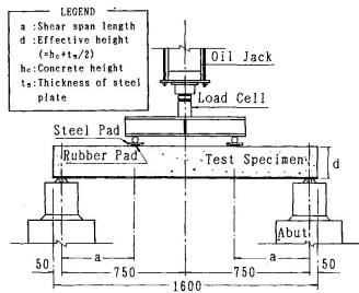
Fig. 2 Two-Point Loading Test Set Up
