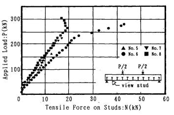
Fig. 8 Tensile Forces at the Body of Studs
