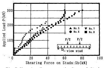
Fig.7 Shearing Forces at the Base of Studs
