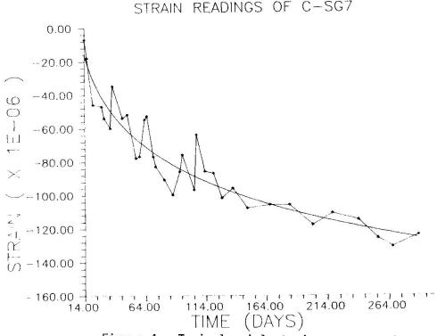
Figure 4 - Typical axial strain measurement.
