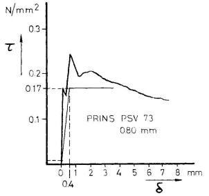
An important feature in this process is the load-slip behaviour and interaction curve for the steel deck used in the composite floor. This load-slip characteristic is typical for each manufacturer's product. In the calculations and experiments the Prince PSV-73 steel decks were used and the load-slip behavior was taken from available literature. See figure 2 on the left.
