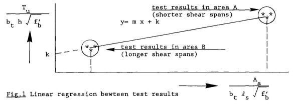
The national regulations of the three countries involved in the research program are based on the 'm and k' method which is related to a linear regression line between test results: y = m x + k (Fig. 1)
