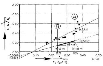
Fig. 3 'Theoretical' and statistical determined (semi-experimental) design function of the profiles examined in the SPRINT-project RA31
