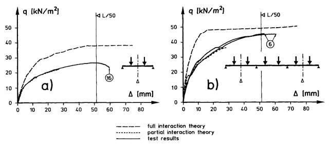
FIGURE 4 Comparison of test and model predictions of load-midspan deflection behaviour. a) simple-span specimen.
