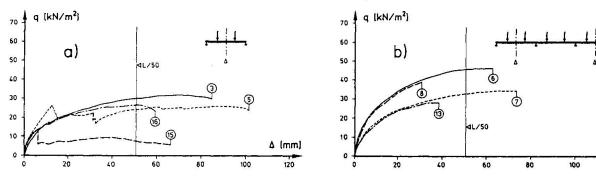
FIGURE 3 Composite slab load-midspan deflection test results. a) Simple span specimens.
