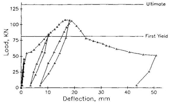
Figure 2: Load vs. Midspan Deflection for SDI-2-1
