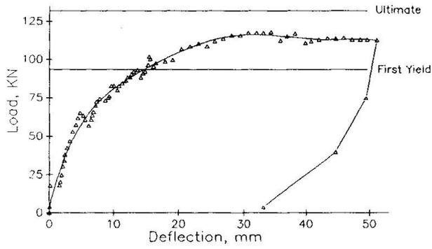
Figure 1: Load vs. Midspan Deflection for SDI-1-1
