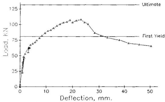
Figure 3: Load vs. Midspan Deflection for SDI-2-2
