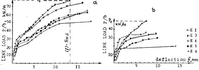
Load-deflection curves for slabs with (a) and without (b) anchor studs.
