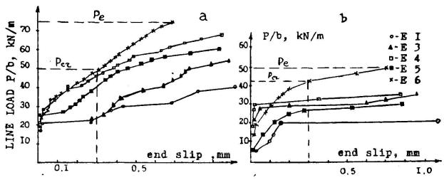
Fig. 5. Load-end slip curves for slabs with (a) and without (b) anchor studs.
