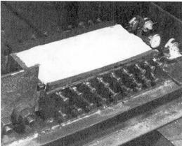
Fig.1. Arrangement (a) and general view (b) of pull-out test I - monolithic concrete block, 2 - steel sheet.
