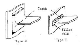
Fig.11 Location of Crack
