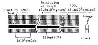
(b) Example of Crack adjacent to Guage Fig.9 Estimation of Initiation of Crack
