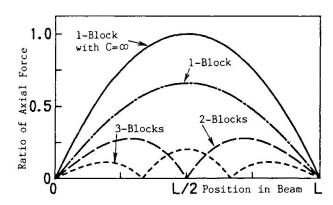
Fig. 3 Axial Force in Slab (C=100MN/m/m)
