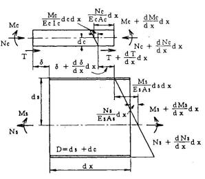
Fig.1 Equilibrium of Forces acting on Elements of Composite Beam
