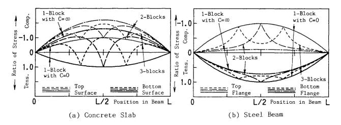
Fig. 5 Axial Stresses (C=1.0GN/m/m)
