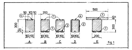
In the elements type D the shear connectors (2) are fixed to the side walls of the casing under an angle of 45°, their cross section being identical with that of dowels (I). The elements of type E are as the elements of type B; but they have a concrete plate of 60 mm thickness.
