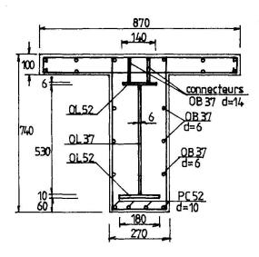
Fig. 2 Section transversale [mm]
