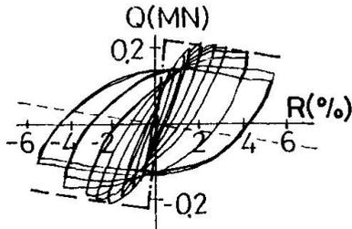
Fig.3 Response of Column Failed in Flexure
