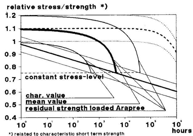
figure 3: stress-rupture and residual strength
