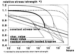
figure 3: stress-rupture and residual strength
