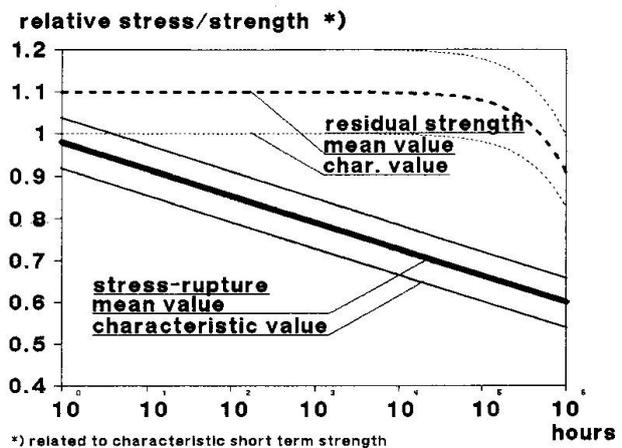
figure 2: stress-rupture behaviour (loaded Arapree) and residual strength of unloaded Arapree
