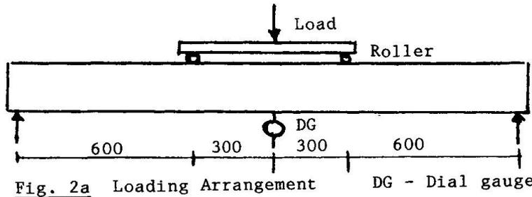
Fig. 2a Loading Arrangement DG - Dial gauge
