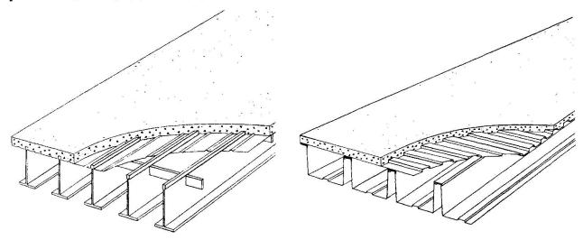
Fig. 3. Long-Span Steel Grid
