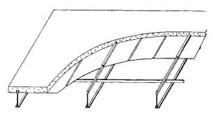
Fig. 2. Steel Grid Floor Systems
