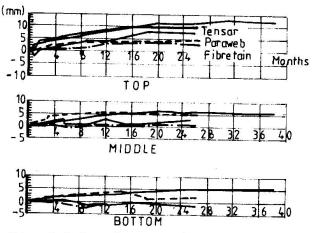
Fig. 5 Outward movement of the facing
