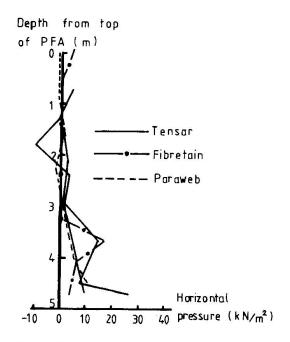
Fig. 3. Lateral pressures on facing
