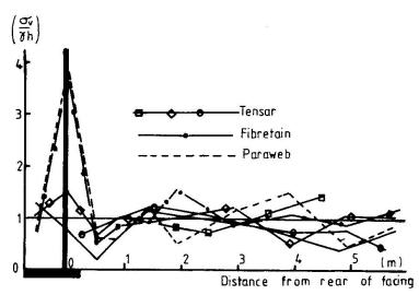
Fig. 2. Vertical pressure on base of PFA
