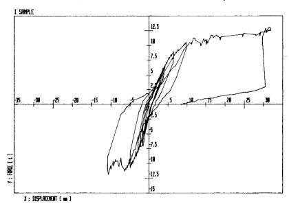
FIG.  $N^{\circ}$  6 - Cyclic tests 2nd set: masonry with braid
