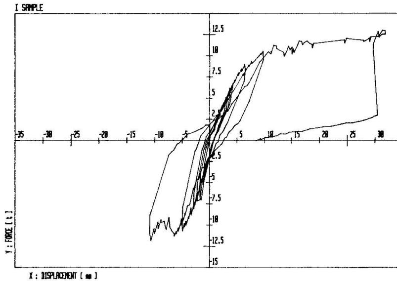
FIG. N° 6 - Cyclic tests 2nd set: masonry with braid
