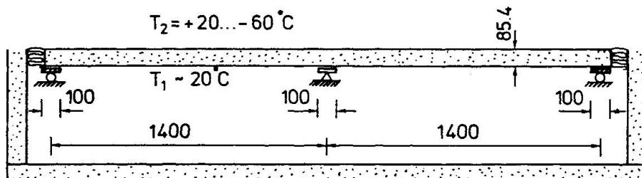
Fig.2. Figurative loading arrangements. Thickness of the steel faces was 0.46 mm, width of the panel 600 mm and the initial shear modulus of the core at  $T = +20^\circ\text{C}$   $4.08 \text{ N/mm}^2$ .
