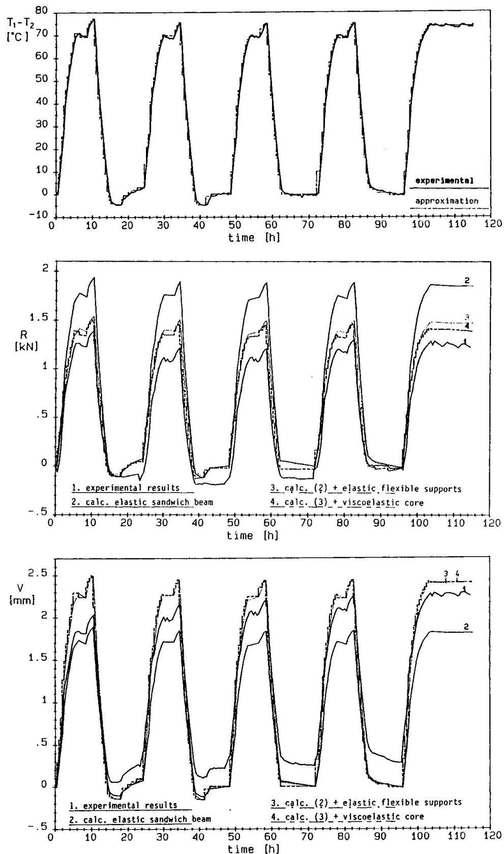
Fig.4. a) Temperature loading history, b) central support reaction and c) deflection in the mid span of the test specimen given in the fig. 2. In the calculations Findley's model was used  $J(t) = 0.2452 + 0.03 t^{0.37}$  ( $\text{mm}^2/\text{N}$ , the time in hours).
