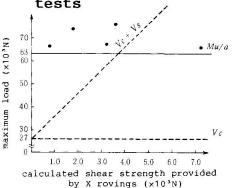
Maximum load vs. calculated shear strength provided by X rovings relationship
