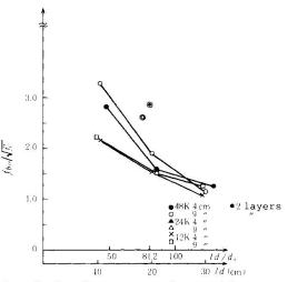
Fig.9 Anchorage strength vs. development length relationship
