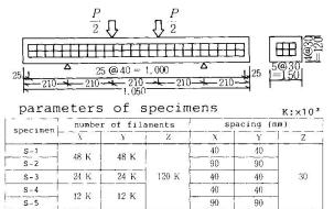
Fig.6 Specimens for the shear tests
