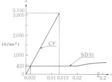
Fig.1 Stress-strain diagram of CF and steel
