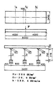
Fig.7 Composite beamr model with three steel girders (unit in mm)
