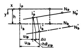
Fig.2 Geometrical relation between plate element and beam element
