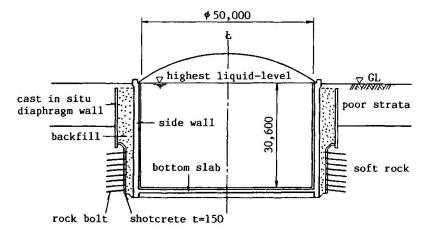
Fig. 1 Cross-section of LPG inground storage tank
