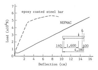
Fig. 3 Load-deflection relationship of specimen
