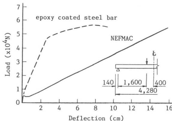
Fig. 3 Load-deflection relationship of specimen
