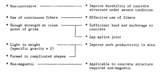
NEFMAC is a new composite material for reinforcing concrete, which is composed of high strength continuous glass and/or carbon fibers impregnated with non-corrosive resin and formed in flat or curved shapes by the filament winding method [1]. NEFMAC has many excellent characteristics as listed in Table 1.
