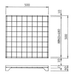
Fig. 7 Reinforcement of new GRC floor tile
