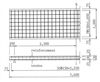
Fig. 9 Tendon and reinforcement of prestressed concrete slab
