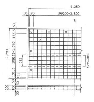
Fig. 4 Reinforcement of fender plate
