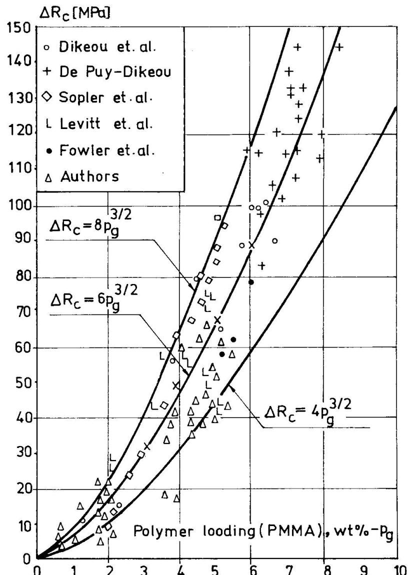
**Fig.1** The dependence between the efficiency of impregnation and the polymer loading
