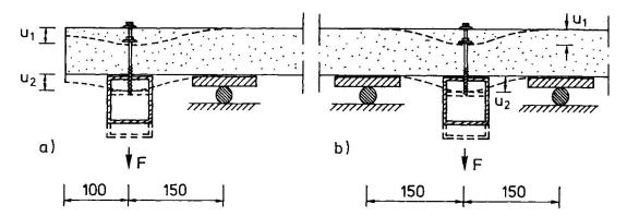
Fig.1. Test arrangements to determinate the tensile stiffness and the strength of a through going screw connection for a sandwich panel with steel faces and a polyurethane core.
