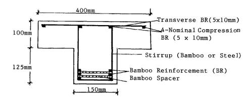
$\underline{\text{Fig. 1}}$  Typical Cross-Section of Beam
