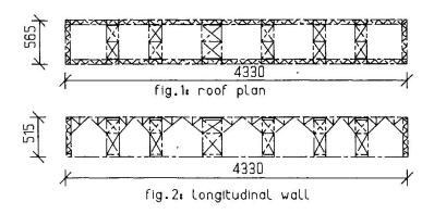
In fact, a three dimensional trussed system is formed by two adjacent frames joined together, both in the vertical plane of the wall and the horizontal plane of the roof (see fig. 3 and fig. 4).
