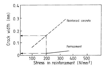
Figure 2 Flexural crack – steel stress behaviour of ferrocement compared with that of reinforced concrete
