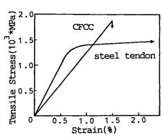
Fig.2 Stress-strain curve
