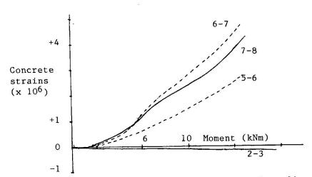
Fig. 4 Concrete strain vs Bending Moment in Beam C6
