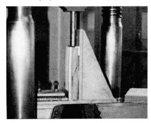
Fig.5 Laboratory testing for shear
