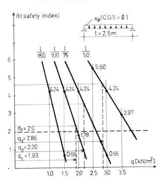
Fig.4 Serviceability limit state for displacement limit
