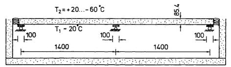
Fig.2. Figurative loading arrangements. Thickness of the steel faces was 0.46 mm, width of the panel 600 mm and the initial shear modulus of the core at T = +20 OC 4.08 N/mm<sup>2</sup>.
