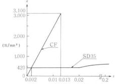
Fig.1 Stress-strain diagram of CF and steel
