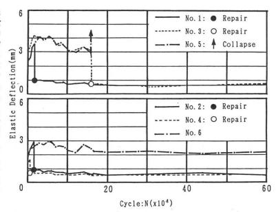
Fig. 1 Relationship between Loading Cycle and Elastic Deflection at Center
