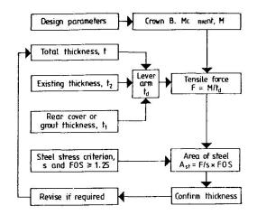
Figure 4 Design procedure
