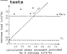
Maximum load vs. calculated shear strength provided by X rovings relationship
