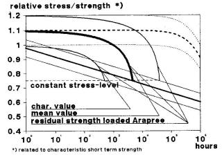
figure 3: stress-rupture and residual strength
