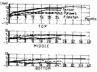
Fig. 5 Outward movement of the facing
