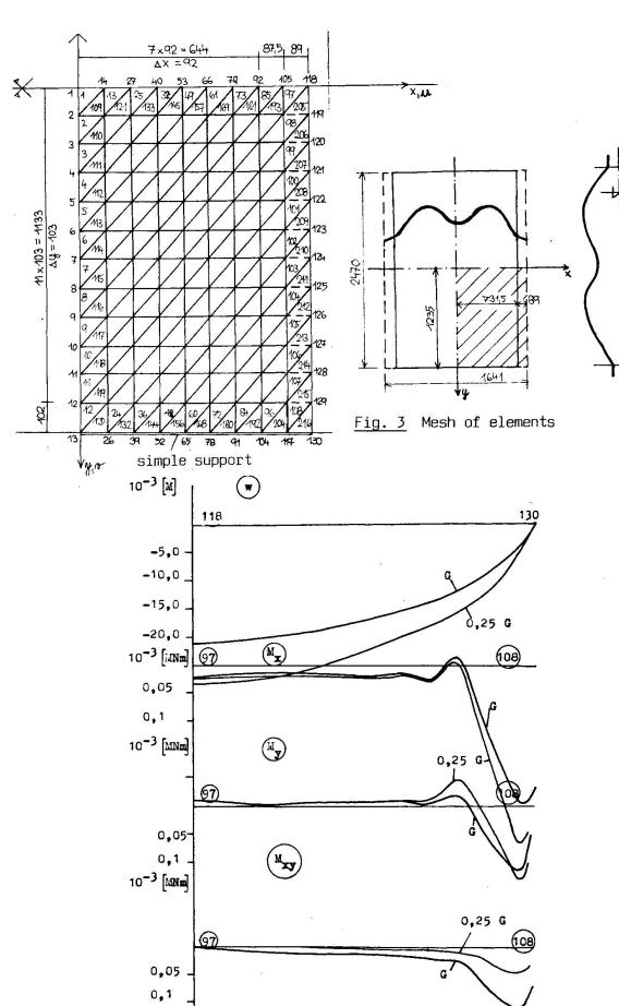
Fig. 4 Shell L9 - displacements and internal forces
