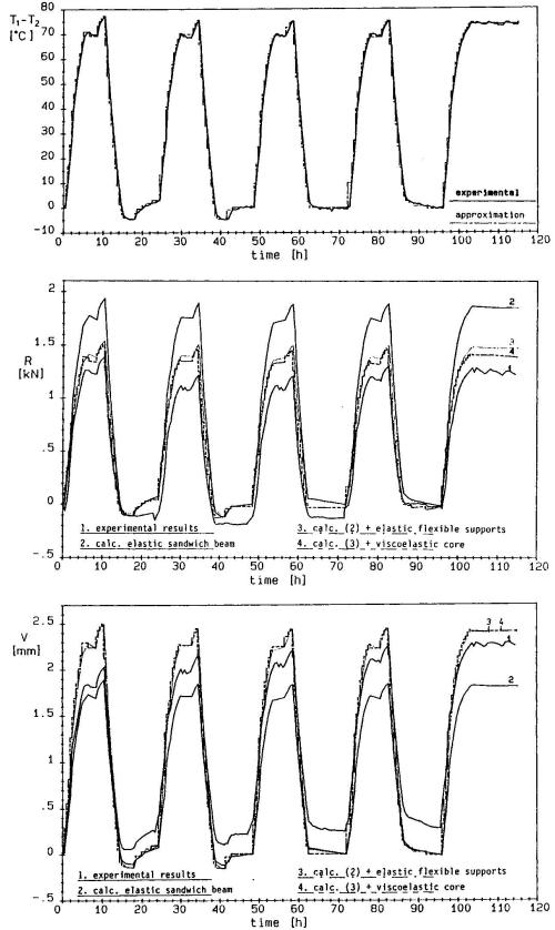
Fig.4. a) Temperature loading history, b) central support reaction and c) deflection in the mid span of the test specimen given in the fig. 2. In the calculations Findley's model was used  $J(t) = 0.2452 + 0.03 t^{0.37} (mm^2/N, the time in hours)$ .
