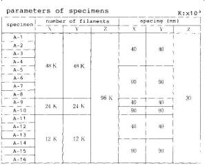
Fig.8 Specimens for the bond tests
