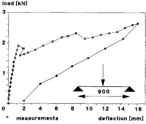
figure 6: load-deflection curve of a concrete panel prestressed with Arapree
