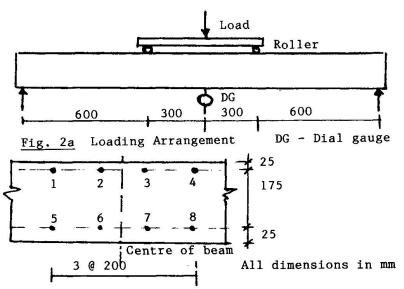
Fig. 2b Part Elevation of Test Specimen
