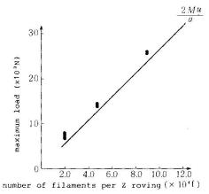
Fig.4 Maximum load vs. the number of filaments per roving in the Z direction relationship
