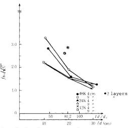
Fig.9 Anchorage strength vs. development length relationship
