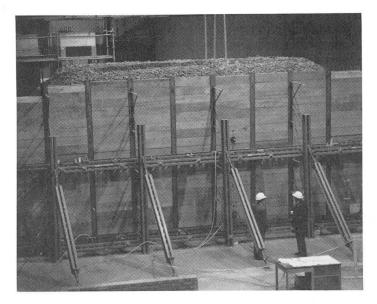
Fig. 1. 'Model' Retaining Wall Apparatus
