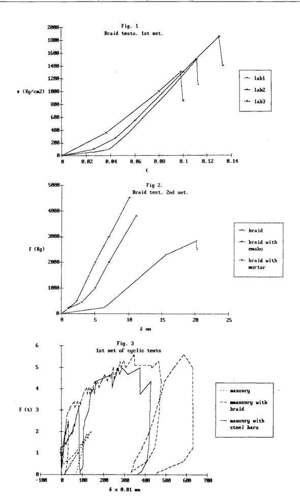
MPa). The samples with emaku show a further improvement in terms of strength, as the bond between the two materials is improved.
