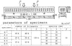
Fig. 6 Specimens for the shear
