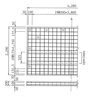
Fig. 4 Reinforcement of fender plate
