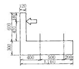
Fig.11 Loading setup
