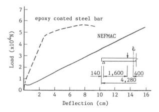
Fig. 3 Load-deflection relationship of specimen
