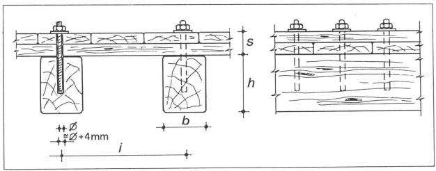
Fig.4 - Transversal and longitudinal cross sections.
