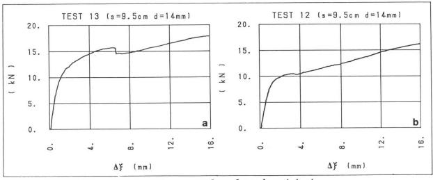
Fig.5 - Some results of push-out test.
