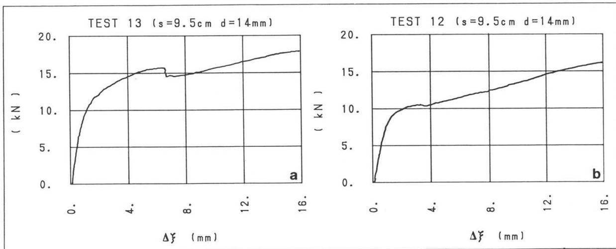
Fig.5 - Some results of push-out test.
