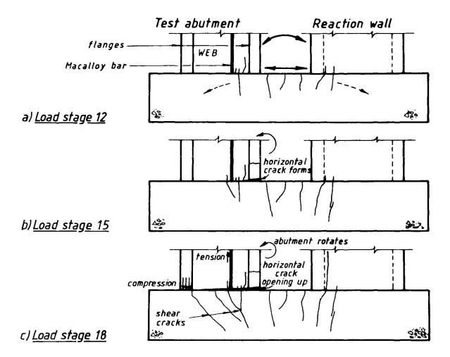
Fig. 3 Development of cracks during testing
