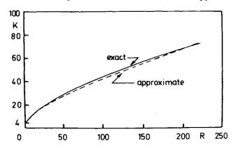
Fig. 4. Accurate and approximate values of the buckling coefficient K
