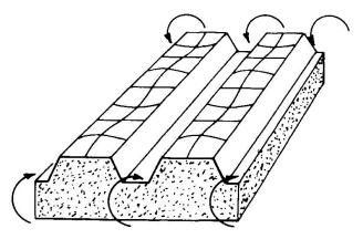
Fig. 1. Typical sandwich panel with a profiled face in compression
