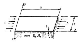
Fig. 2. Plate element in compression with core support
