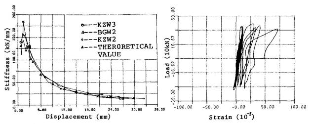
Fig. 6 Stiffness Degradation
