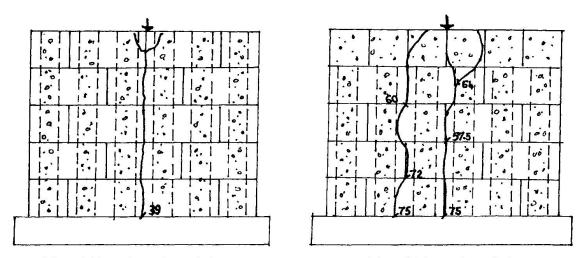
wall without a bond beam wall with a bond beam Fig. 2 Crack pattern of the reinforced walls
