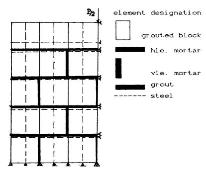
Fig. 4 Idealized model for a wall with a bond beam.
