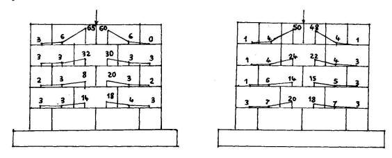
wall without a bond beam wall with a bond beam Fig. 3 Vertical strain distribution in the reinforced walls
