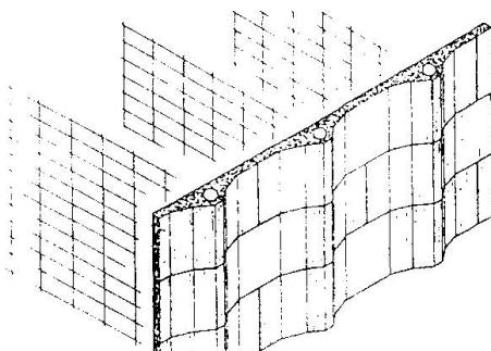
Fig. 5 - STRUCTURE: BÉTON/TREILLIS
