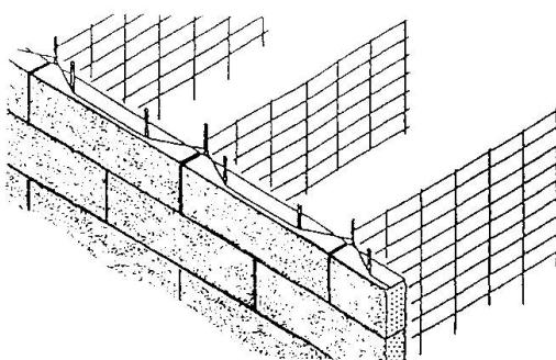
Fig. 7 - STRUCTURE: BÉTON/TREILLIS
