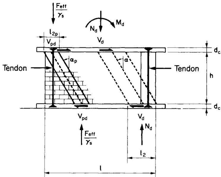
Fig. 4 : Design of prestressed masonry shear wall.
