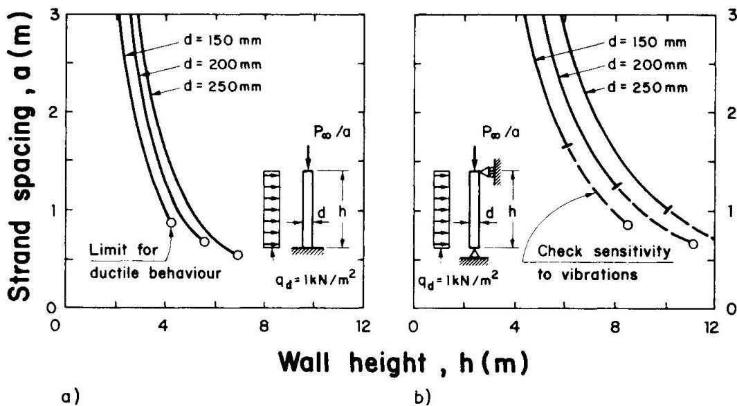
Fig. 3 : Diagrams for the preliminary design of laterally loaded walls:
