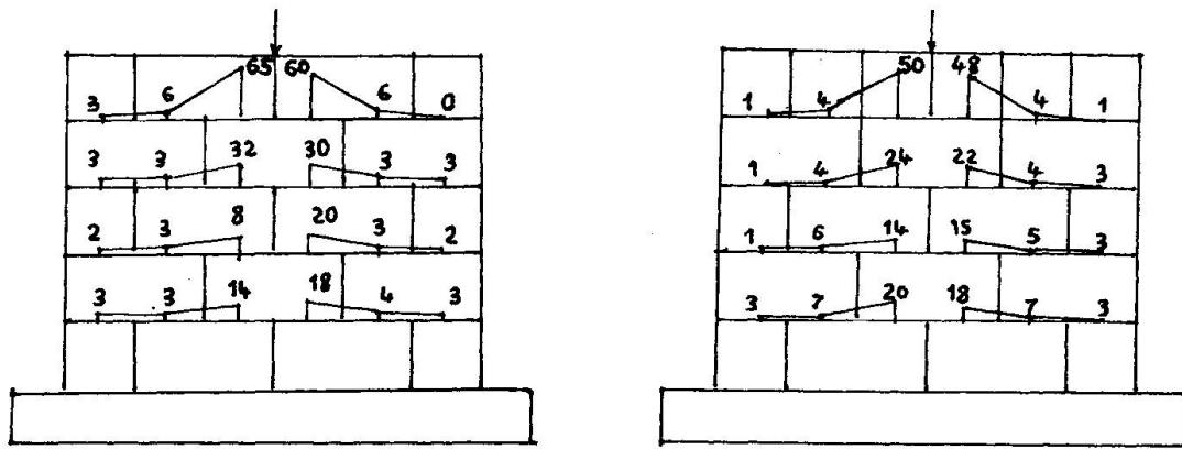
Fig. 3 Vertical strain distribution in the reinforced walls
