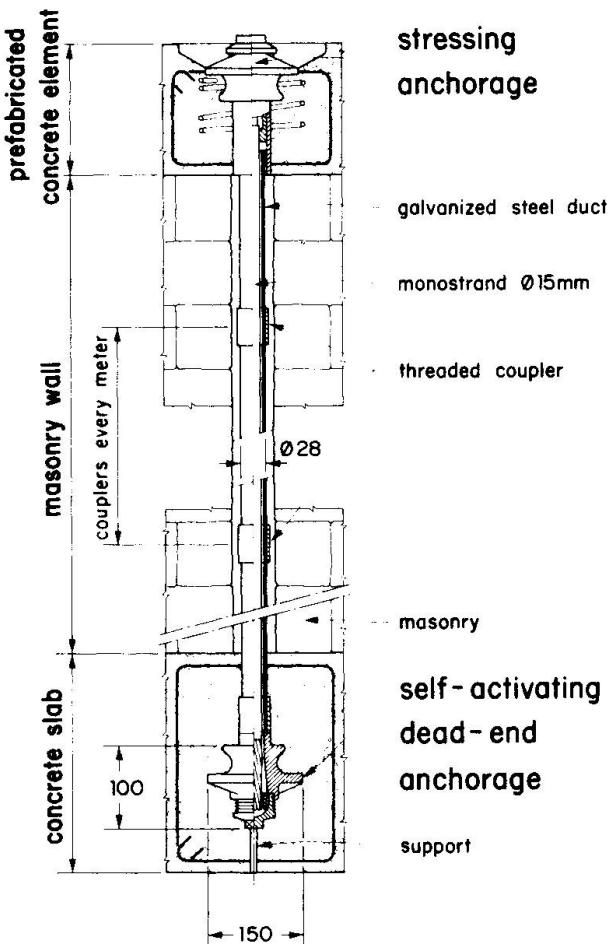
A new post-tensioning system for masonry walls has recently been introduced in Switzerland, [4, 5]. For an optimum corrosion protection by grease and polyethylene sheathing as well as for constructability an unbonded monostrand system has been used. A typical tendon for post-tensioned masonry is illustrated in Fig. 1.
