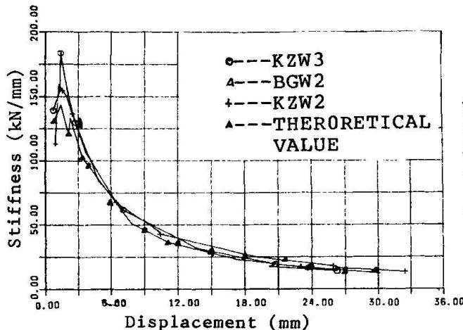
Fig.6 Stiffness Degradation
