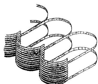
Fig. 4 - STRUCTURE: TÔLE/ÉTRIERS
