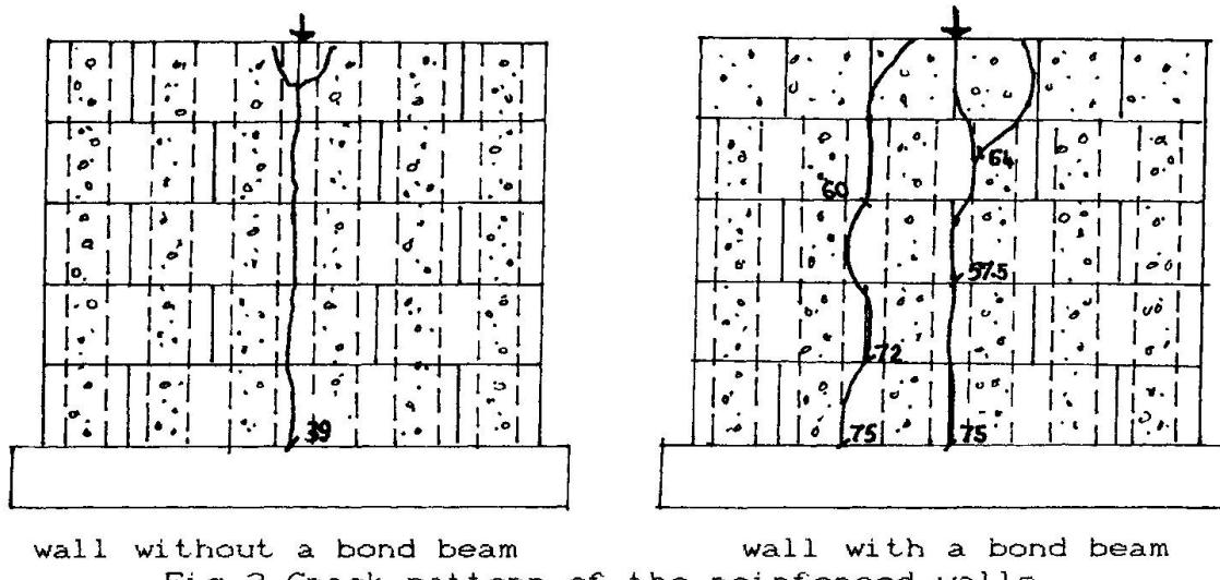
Fig. 2 Crack pattern of the reinforced walls
