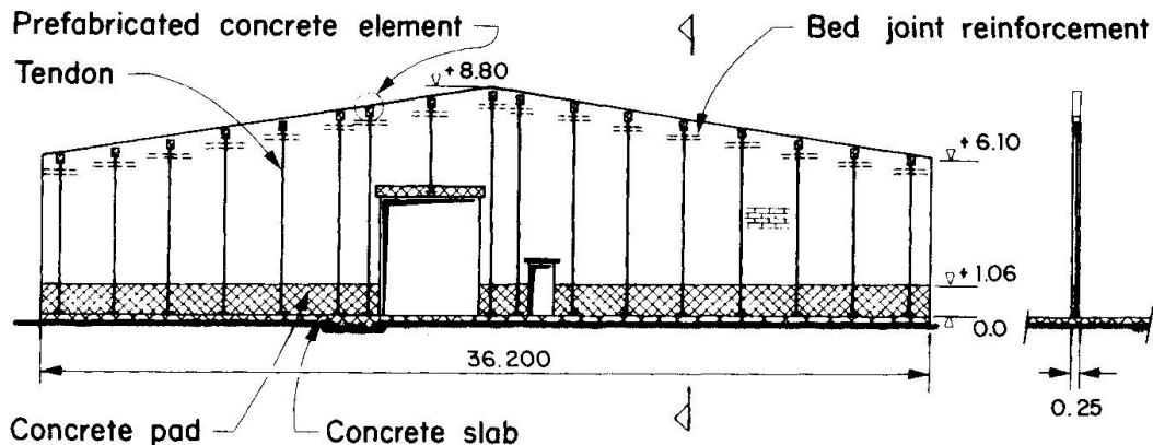
**Fig. 6 : Post-tensioned masonry wall in factory.**
