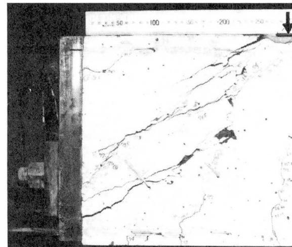
Fig.4 Ultimate state of the shear test specimen
