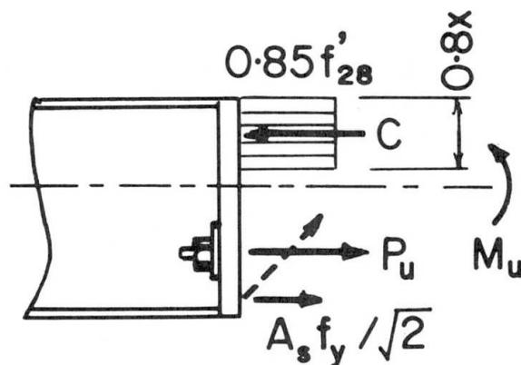
Fig.3 Theoretical model for estimating bending strength
