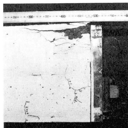
Fig.2 Ultimate state of the bending test specimen
