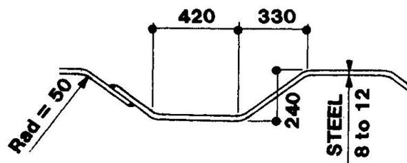
Fig 2 : Typical cross section of corrugated web
