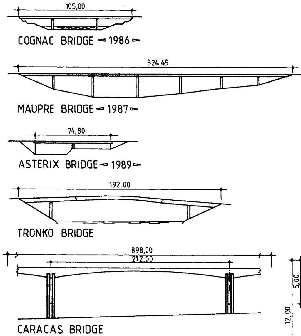
Fig 5 : Examples of bridges with corrugated webs
