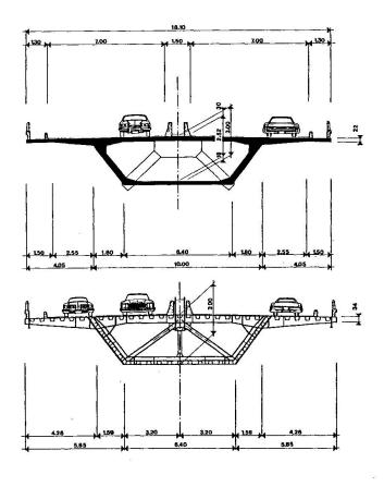
Fig. 3 Concrete and steel cross-sections of the deck
