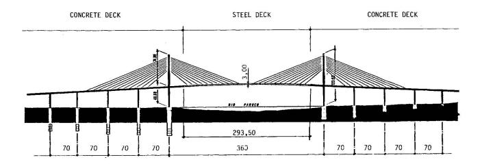
Fig. 1 Elevation of the Bridge
