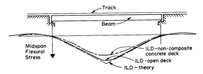
Figure 1 - Influence lines for a simply-supported stringer supporting railway
