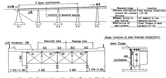
Fig. 6 Measuring plan for Toyoda Viaduct
