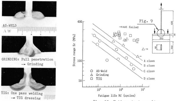
Fig. 9 Macro-Etch results of specimen
