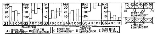
Fig. 13 Comparison of axial force in diagonal members of a cross bracing
