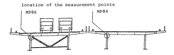
Figure 1: Cross-section of a steel bridge with transverse bracing
