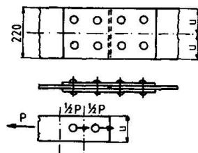
Fig. 5 Configuration of the investigated example with loaded rivets.
