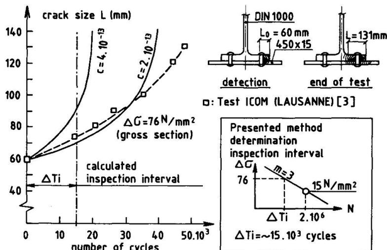
Fig. 11 Influence change of the constant C. Comparison theoretical crack growth with test results.
