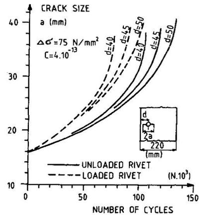
Fig. 6 Crack growth curves. Comparison between loaded and unloaded rivets. Influence of different edge distances.
