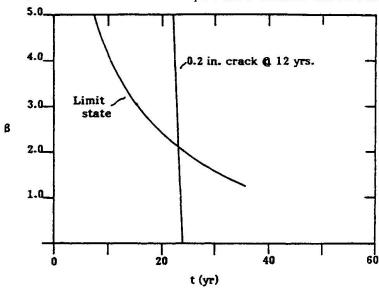
Fig. 3 Updated reliabilities for the Yellow Mill Pond Bridge when a 5 mm crack was found in the first inspection after 12 years of service.
