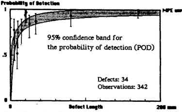
Fig. 1 Inspection reliability for MPI
