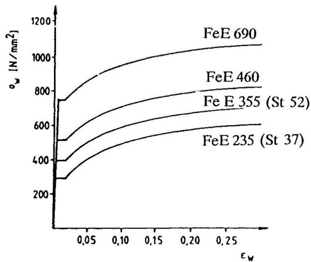
Figure 4: True stress-strain-curve
