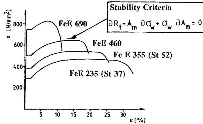
Figure 3: Technical stress-strain-curve
