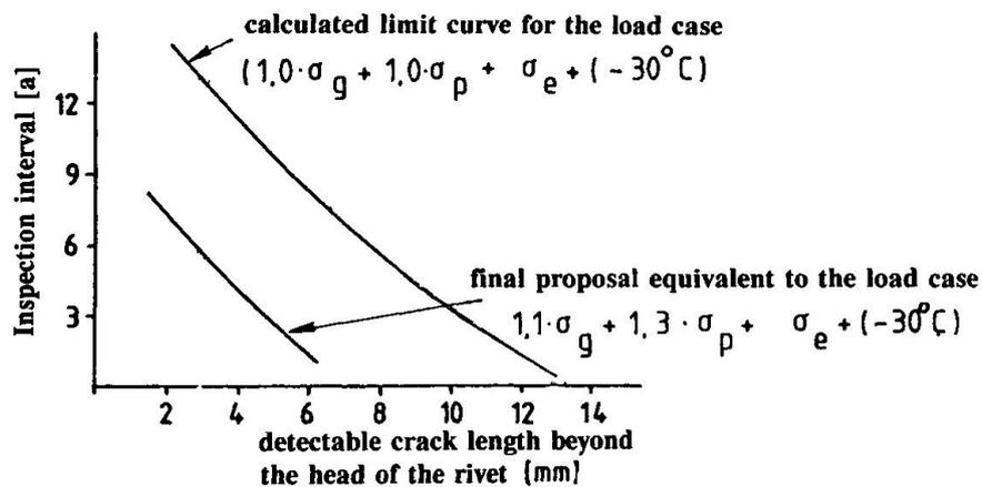
Figure 25: Crack propagation behaviour and inspection interval
