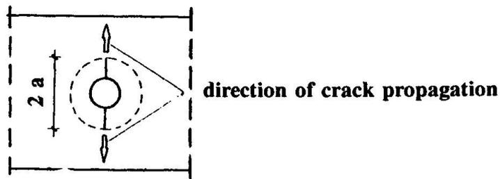
Figure 20: Definition of the starting crack size
