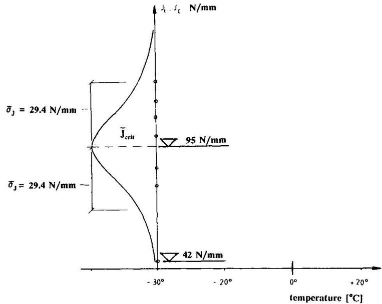
Figure 13: Critical material resistance values  $J_{crit}$  obtained from small scale test specimens
