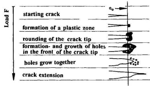
Figure 12: Procedure of crack propagation
