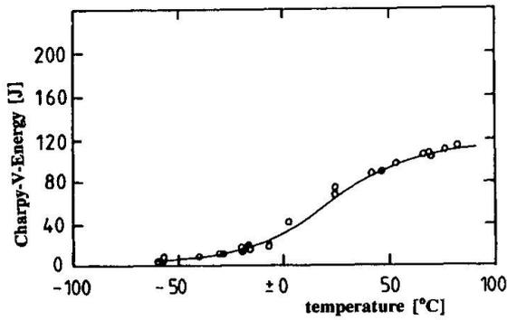
Figure 16: Charpy-V-energy-temperature curve
