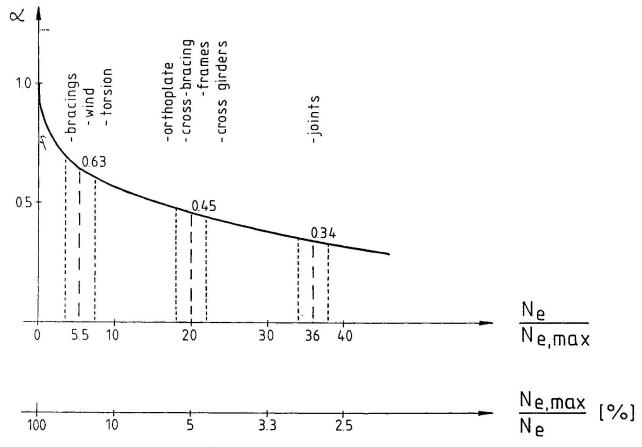
Fig. 7 Fatigue load factor for different details
