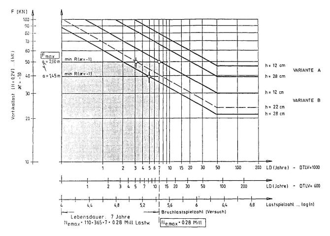
Fig. 5 Fatigue strength curve expansion joint
