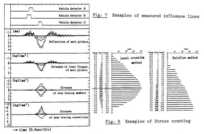
the repeated stresses induced by relative vertical deflections between adjacent main girders and by deflections of concrete slabs.
