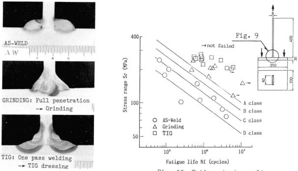
Fig. 9 Macro-Etch results of specimen
