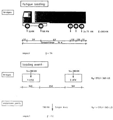
Fig. 2 Fatigue loading for bridges and expansion joints
