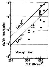
Fig 2 Relationship between crack growth rate da/dN and △ K of wrought iron.
