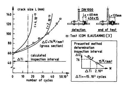
Fig. 11 Influence change of the constant C. Comparison theoretical crack growth with test results.
