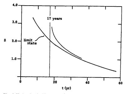
Fig. 4 Updated reliabilities for a W30×360 rolled section.
