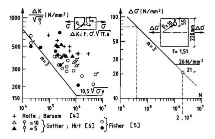
Fig. 9 Relationship  $\Delta K/\sqrt{p}$  versus fatigue life, and SN-curve of crack initiation.
