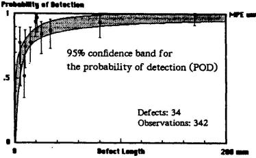
Fig. 1 Inspection reliability for MPI
