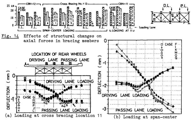
Fig. 15 Effects of structural changes on floor slab deflections
