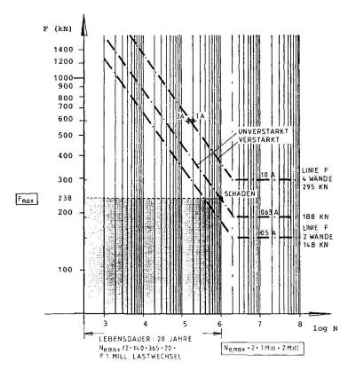
Fig. 4 Fatigue strength curve bracing
