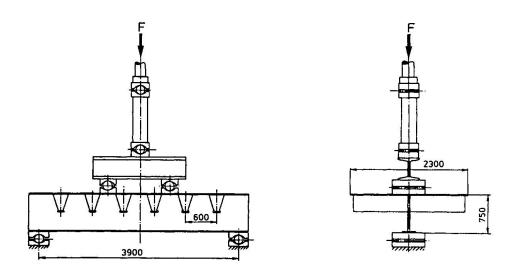
Fig. 1 Testing performed
