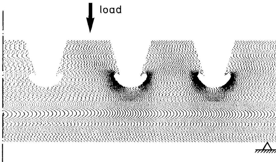
Fig. 2 Global stress distribution in one half of the web loaded as in Fig. 1
