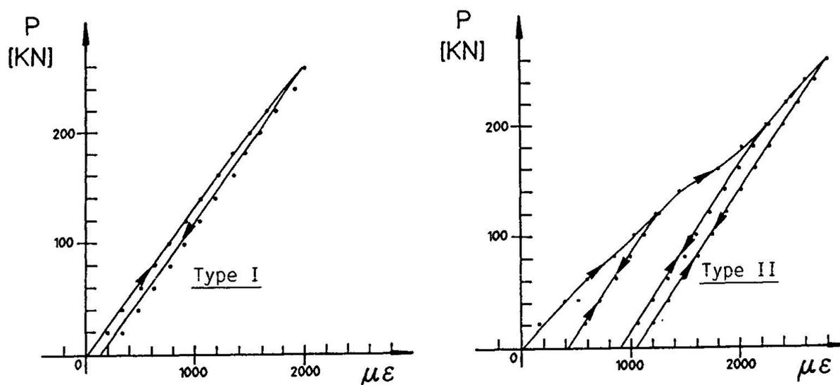
Fig. 7 Load-strain diagrams of the relaxation tests on type B specimens
