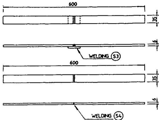
A number of 62 specimens have been tested: 31 with S3 weldings and 31 with S4 weldings.
