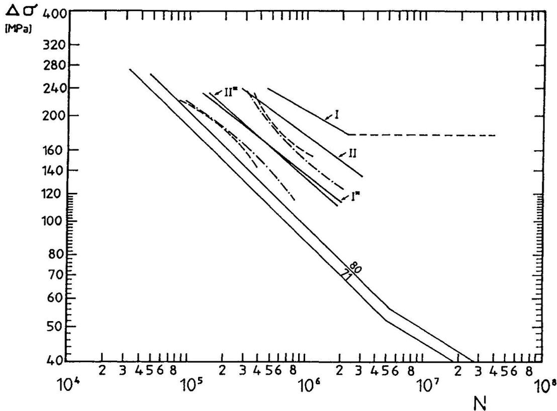
Fig. 12 Comparison between experimental results and ECCS curves
