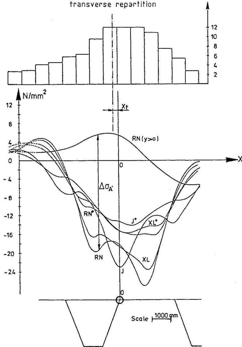
Fig 6 :  $\sigma_D$  Influence lines for a wheel (axis1 ;  $y=0$ )
