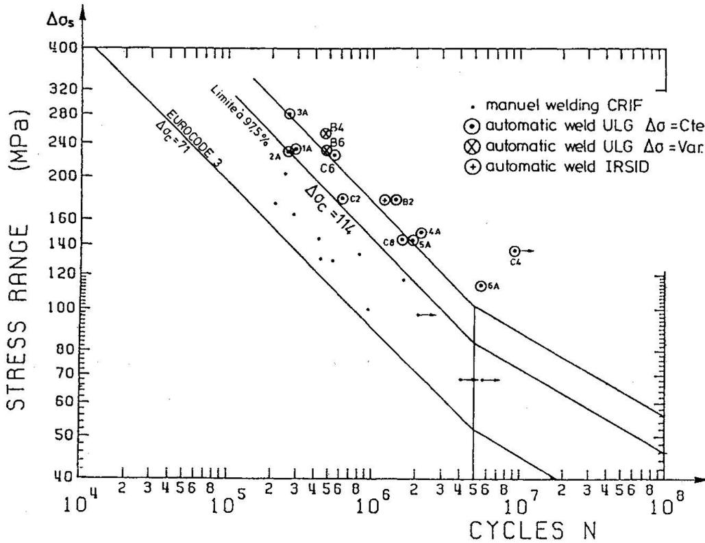
Fig.9: Crack initiation at the weld root: Δσ<sub>s</sub>
