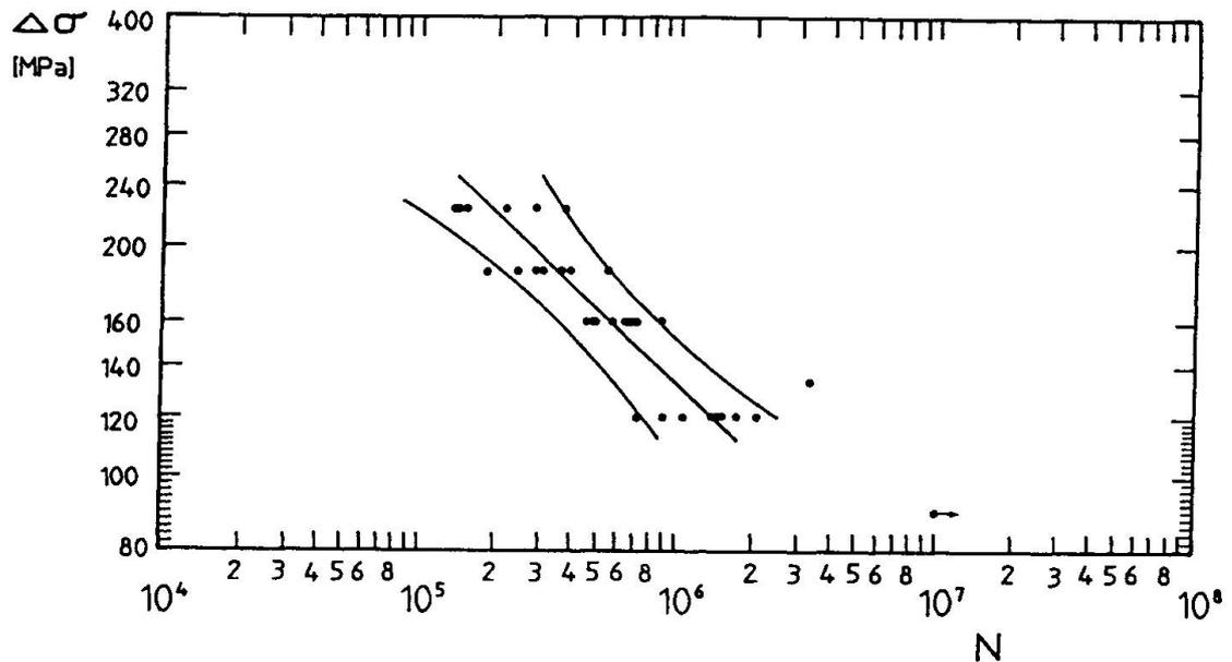
Fig. 10 Fatigue results on S4 welding specimens
