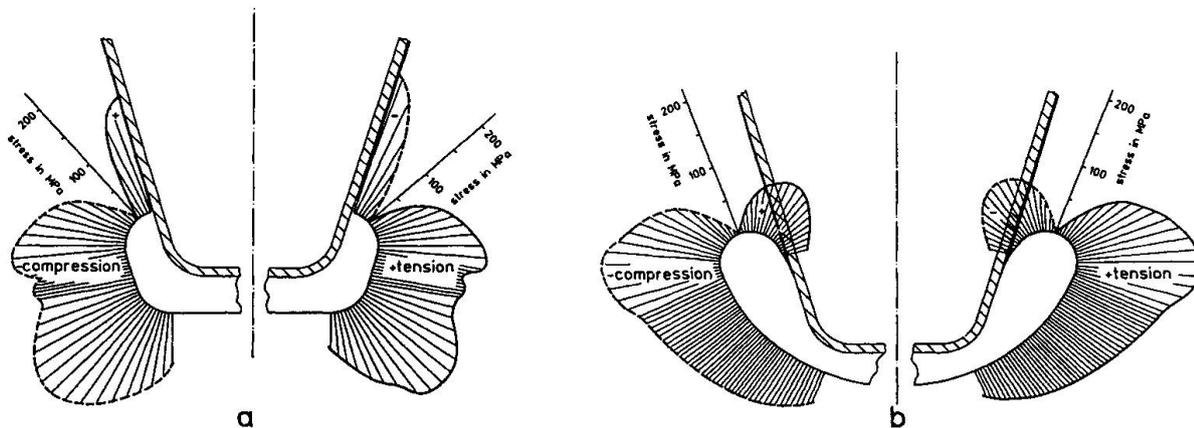
**Fig. 5** Stress distribution along the edges of the cut-outs of the commonly used (a) and the new (b) shape
