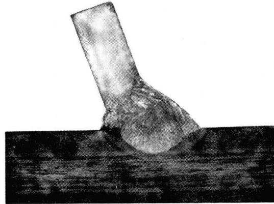
Fig.2 : Macrograph of the weld
