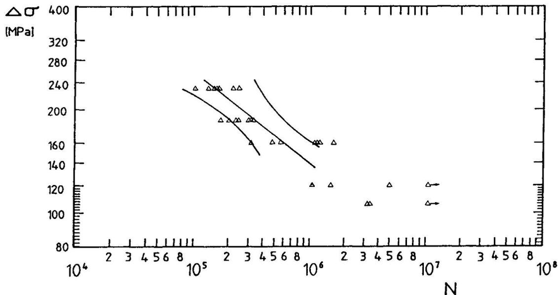
Fig. 9 Fatigue results on S3 welding specimens
