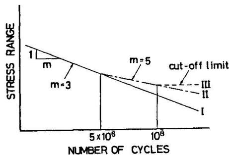
Fig.4 S-N diagram used for fatigue damage analysis
