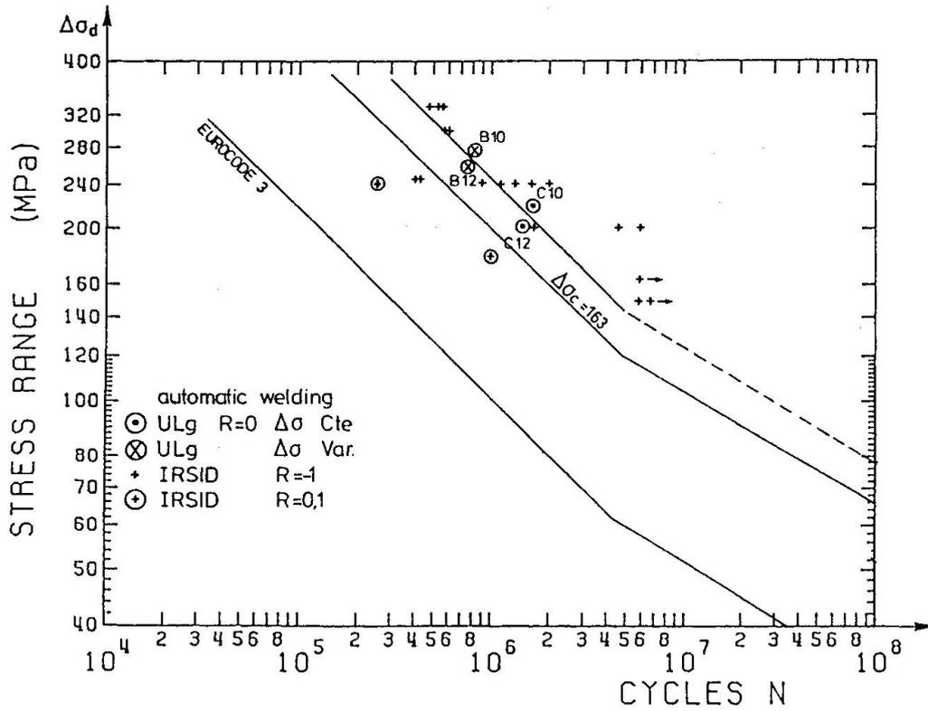
Fig.8: Crack initiation at the weld toe : Δσ<sub>d</sub>
